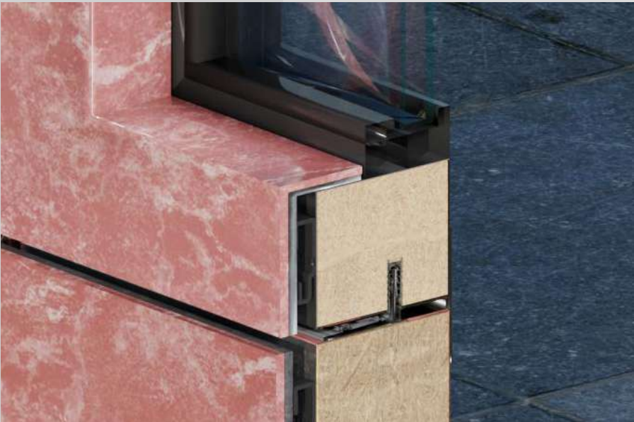
VERTICAL WINDOW section
