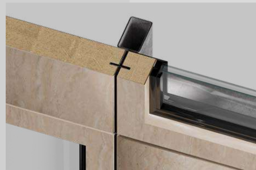
HORIZONTAL WINDOW section
